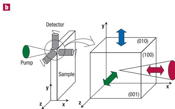
**Figure 4** Lasing in three dimensions. a, Lasing spectra measured in the three orthogonal directions, *x*, *y* and *z*. The inset shows the spatial distribution of laser emission in the pump direction (*x* direction). b, The configuration used in measurements and schematics of (100), (010) and (001) planes of BPII and directions of laser emission (arrows).
