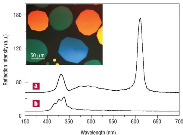
**Figure 2** Reflection spectra of the liquid crystal/chiral dopant mixture E48:CB15 (1:1.25 v/v%). Curve a, BPII single crystals at 24.6 °C. Curve b, The helical state at 21.0 °C. The inset shows a micrograph of the BPII single crystals growing from the isotropic fluid phase (dark region). The micrograph was produced with a digital camera (MagnaFire-SP, Optonics) mounted on a polarizing microscope (Nikon Optiphot-Pol).
