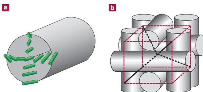
**Figure 1** Schematic of the BPII structure. **a**, The director field inside a double-twist tube. **b**, Stacking of double-twist tubes and unit cell (red) and disclination lines (black). The unit cell is bounded by six planes that bisect the double-twist tubes. Disclination lines start at the centre of the unit cell, and continue to those four corners where the three nearest double-twist tubes in the unit cell form a coordinate system with the same handedness as the liquid crystal.
