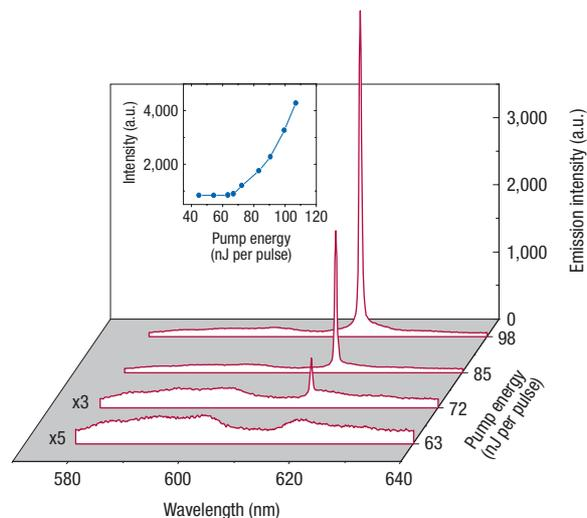
**Figure 3** Fluorescence and lasing spectra at different pump energies. The inset shows the emitted intensity at a wavelength of 617.23 nm versus pump energy. The first two spectra are shown at x5 and x3 magnification for clarity.
